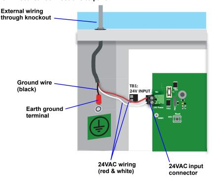
3. Secure the incoming electrical service wires to the Liqui-tect panel's 24VAC input by sliding the wires into TB1, the 24VAC input terminal block. There is no polarity requirement when connecting to TB1. The ground wire must be connected to the earth ground terminal located on the side of the panel (see **Figure 5**).
